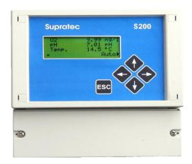
The S200 displays the concentrations of the parameters measured by STAC2 and the models used to determine these concentrations. It also allows to recover data from 2 parameters on 4-20 mA outputs
